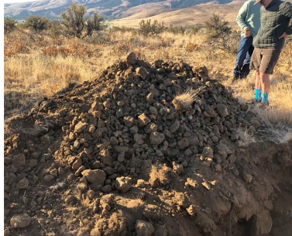
Test pit spoils.
